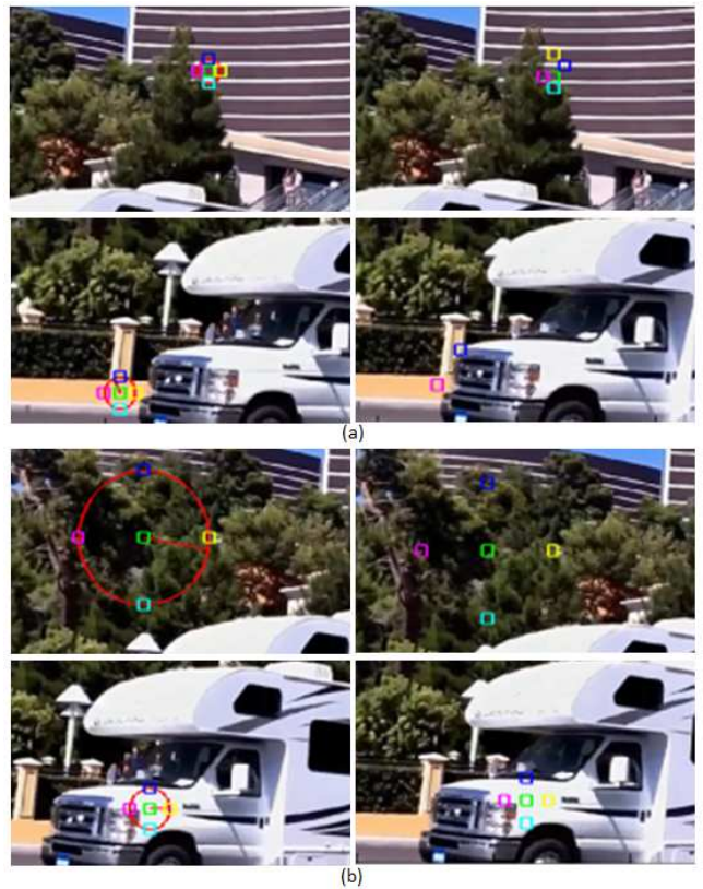
Fig. 3. Example of motion vectors: (a) motion vectors without consistency, and (b) motion vectors with consistency.
